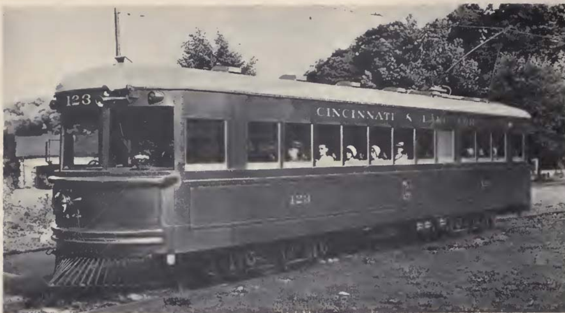
One of the new cars. Note the low height, tapered ends and curved roof specially designed for high speed operation
